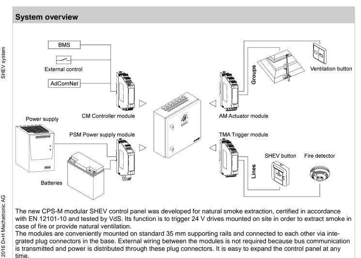
The new CPS-M modular SHEV control panel was developed for natural smoke extraction, certified in accordance with EN 12101-10 and tested by VdS. Its function is to trigger 24 V drives mounted on site in order to extract smoke in case of fire or provide natural ventilation.
